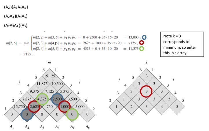
The optimal cost is entry m[1,6] = 15,125. Recovering the actual parenthesis structure requires the use of this recursive algorithm:
