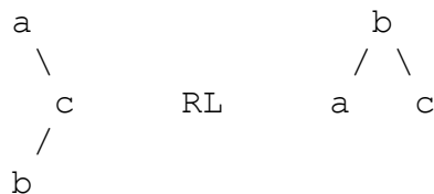
Figure 10 (balanced Figure 9 AVL tree)
