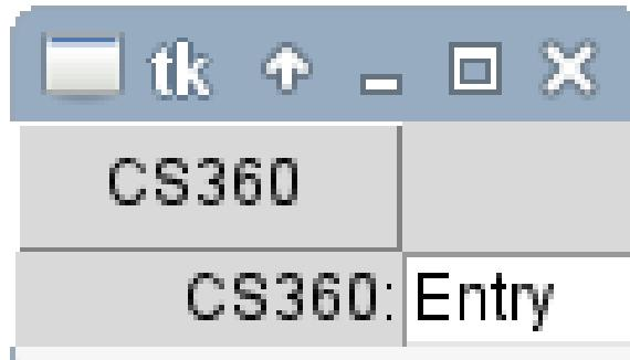
Pressing the CS360 button should toggle the Entry box between displaying 'CS360' and 'Python'. 'Entry' is displayed in the Entry box only when the application is first launched.
