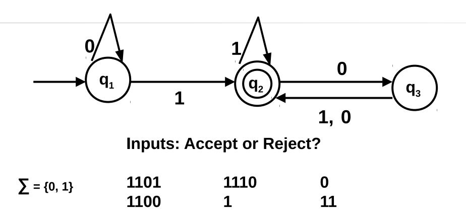
Set of all strings (A) accepted by a machine (M) is the *Language of the Machine* M *recognizes* A or M *accepts* A
